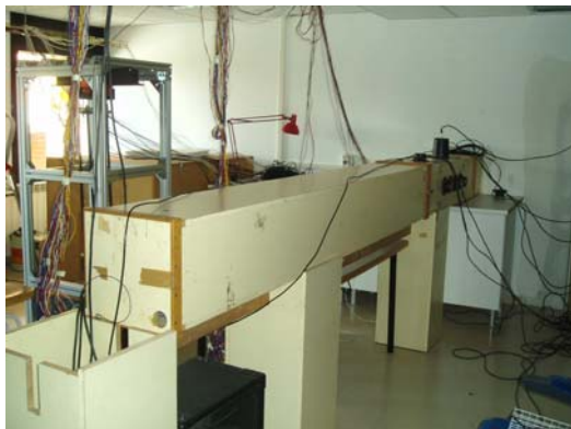
Figure 1: Acoustic tube connected to the anechoic room.
